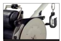
**4. Press-arm** Automatic press-arm for self-hauling
